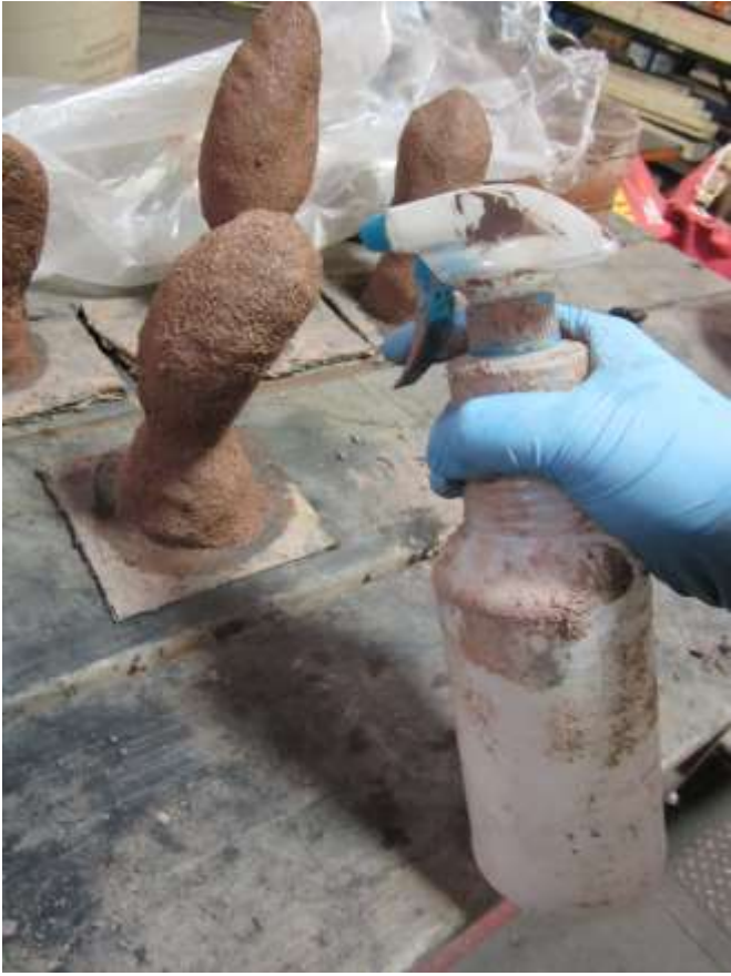
Spraying the mold with water before adding the next layer.
