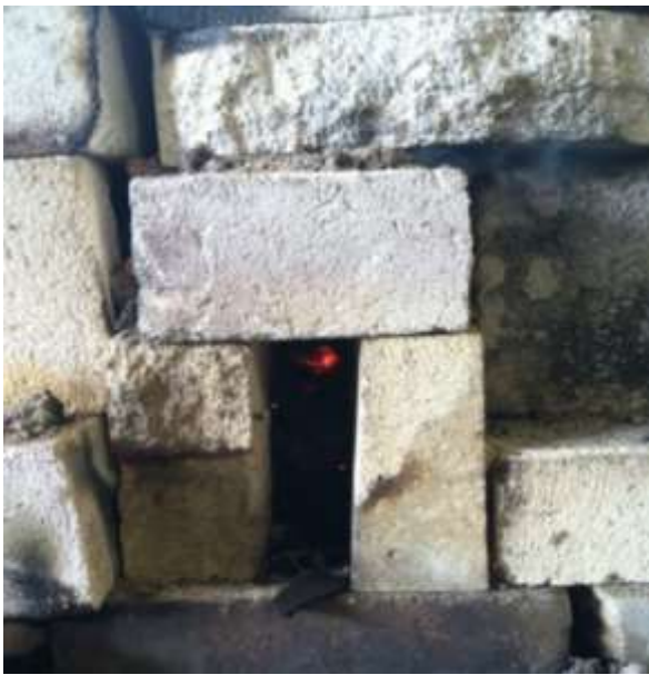
The tuyere left for the pipe to fit into.
