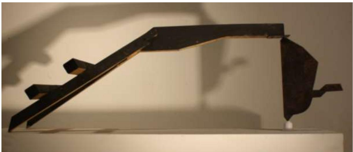
Uma is Japanese for “horse”, and it is what holds the sweep upright as it’s rotated. There is no defined shape for the Uma, but it must be able to hold the sweep on its axis while it is rotated around. This can be as simple as a steel plate with a hole in it held over the sweep by a wooden apparatus. The Uma should be designed in a fashion that is convenient for you. An example is shown above.
